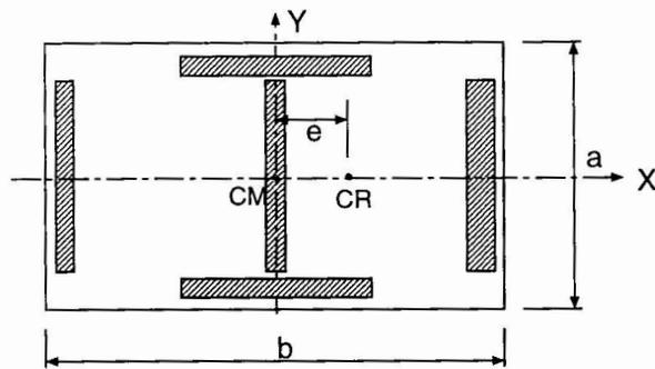
Fig. 1: Plan view of a 5-plane single storey monosymmetric building model
