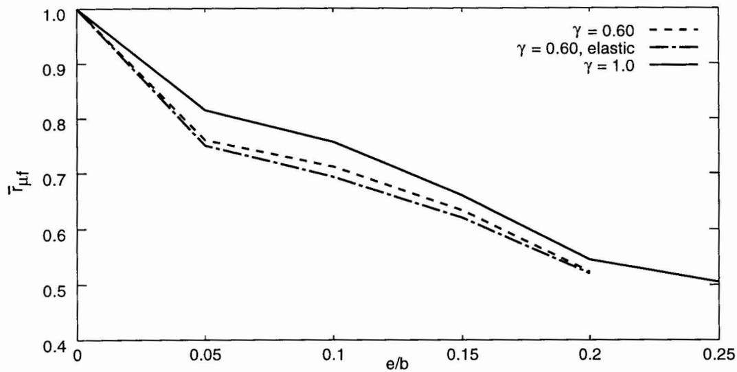
Fig. 2a: Ratio of flexible edge ductility demands,  $\Omega_R = 1.0$
