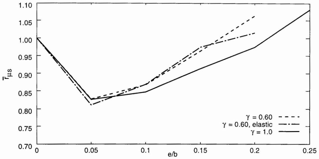
Fig. 3a: Ratio of stiff edge ductility demands,  $\Omega_R = 1.0$
