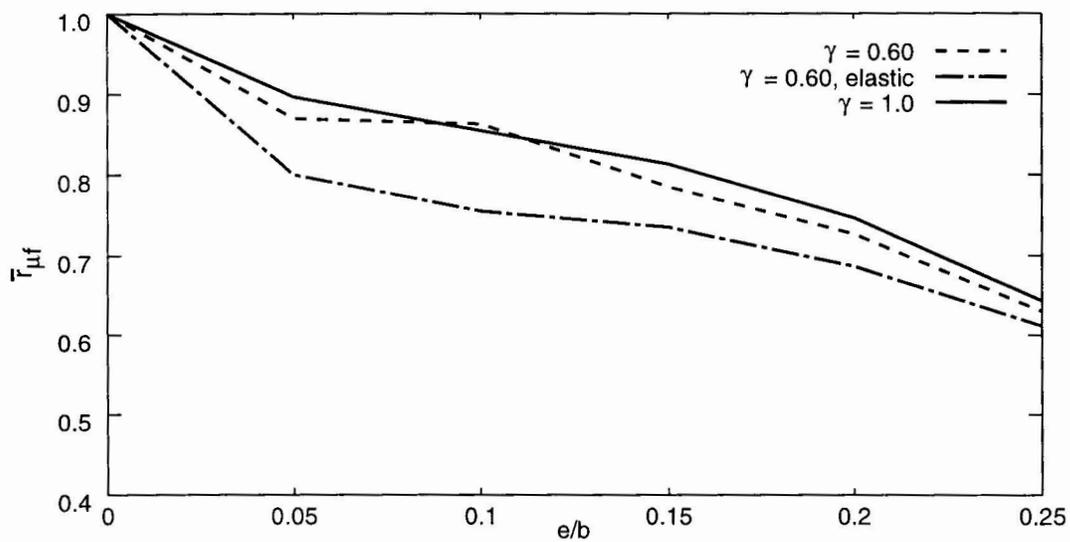
Fig. 2b: Ratio of flexible edge ductility demands,  $\Omega_R = 1.25$
