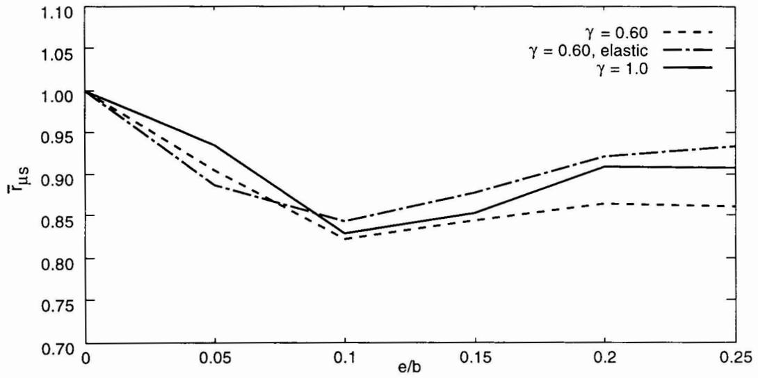
Fig. 3b: Ratio of stiff edge ductility demands,  $\Omega_R = 1.25$
